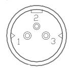
Pin 1: Vcc Pin 2: GND Pin 3: PD
